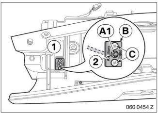
Insert branch **A1** in the glove compartment (1) and secure it to mounting plate **B** with a knurled nut (2).
